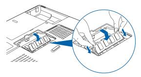
Figure 4-12. Installing a Memory Upgrade Module
